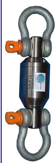
The Elkins EE-1 EE-2 & EE-3 swivels features a rotating spindle which is located exactly within twin needle roller bearings with the inline forces being carried independently via a single heavy duty thrust race. The complete assembly is oil filled and due to its unique pressure balanced system can ensure freedom of movement even at the greatest ocean depths.
