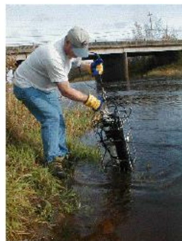
ISUS Nitrate sensor in a Water Quality Monitor application.
